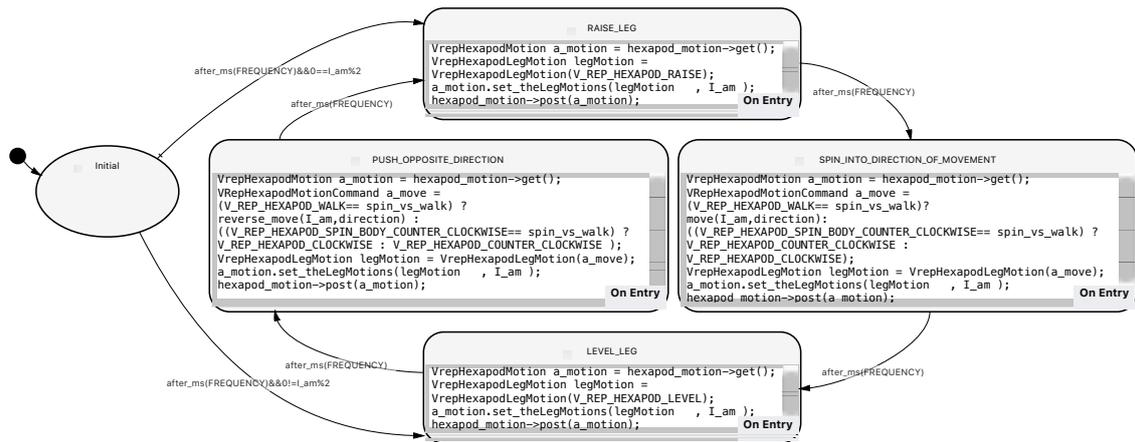
Figure 4: Executable model (as a parameterised LFLSM) for each leg of an  $n$ -legged robots. We can compose the walking gait at any direction and also the spinning (clockwise or counter-clockwise) gait.
