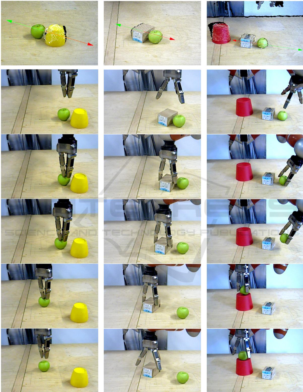
Figure 11: Execution results of three different scenarios: “pushing” (left), “pick and place” (middle), and “put on top” (right). The top row shows the results of the geometrical reasoning. The allowed direction is marked with a green arrow, the forbidden one with a red arrow. The full scene is also shown in the video attachment of the paper.
