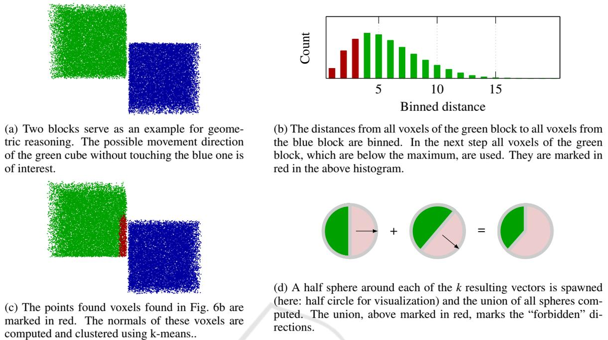
Figure 6: Step-by-step explanation of the geometric reasoning algorithm.
