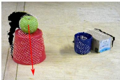
Figure 8: Qualitative results for the geometrical reasoning method. The algorithm is applied to the object pair apple and red pedestal. For graphical purposes only the largest cluster is shown with a red arrow. The computational steps for the arrow are detailed in Fig. 6d. Here, the arrow points from the apple downwards to the pedestal, which is the “forbidden” direction.
