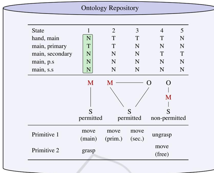
Figure 3: This figure shows one example action, pick and place, in the proposed ontology repository, which is also shown in Fig. 2b. It consists of three parts: the SECs (top), including the SEC precondition (top with green bar), topological preconditions (middle), and primitives (bottom). “M” is the main object; “O” depicts other objects in the scene, and “S” stands for support.
