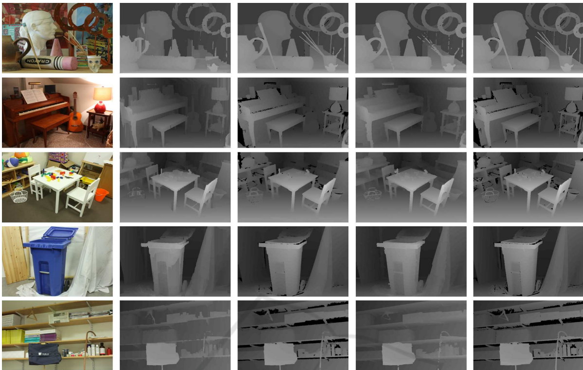
Figure 7: Results on the new Middlebury training set for (a) ArtL. (b) Piano. (c) Playtable. (d) Shelves. From left to right: Reference image, disparity maps produced by (Mukherjee and Guddeti, 2014), (Liu et al., 2015) and ours, respectively. Finally ground truth disparity maps.
