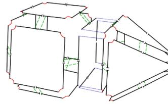
Figure 2: Two darts sewed by  $\alpha_0$  link form an edge (black lines). Several edges sewed by  $\alpha_1$  links (red curves lines) form a face. Several faces sewed by  $\alpha_2$  links (green large dotted lines) form a volume. Several volumes sewed by  $\alpha_3$  links (blue thin dotted lines) form one connected component.
