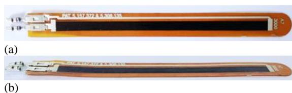
Figure 1: (a) Top and (b) lateral view of a resistive flex sensor, manufactured by Flexpoint Inc.
