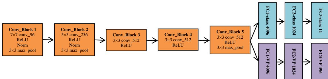
Figure 1: The CNN Architecture. ReLU is the activation function we use. Max-pooling is used in the first, second, and fifth convolutional blocks. Fully connected viewpoint output layer is an object category dependent layer. Fully Connected layers (FC) are followed by a dropout layer with rate 0.5.
