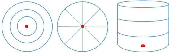
Figure 2: Descriptor spatial partitioning: 3 circles, 8 sectors, 3 sections. Projected center of gravity is shown in red.
