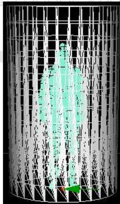
Figure 1: 3D spatial partitioning in 12 sections. Projected center of gravity is shown in red, fixed point view direction is shown by a green arrow.
