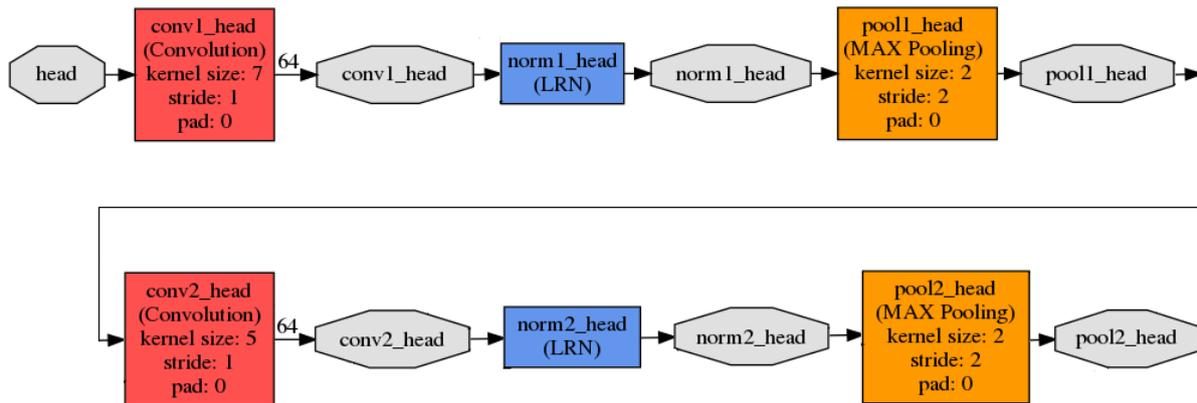
Figure 2: DCNN used to learn the head feature matrix,  ${}^hF^p$ .
