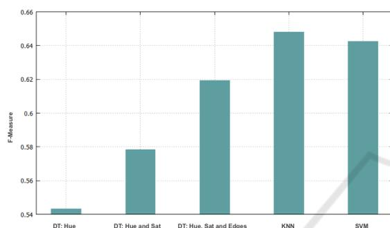
Figure 8: F-measure average obtained in the recognition of apple pixels. First it shows the improvement of using three characteristics with tree decision and then the comparison using KNN and SVM.
