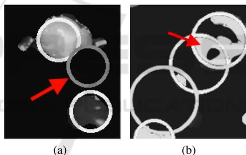
Figure 7: Wrong circles detected because the higher region presents an outward circular curve or because a region exhibits circular gaps inside.
