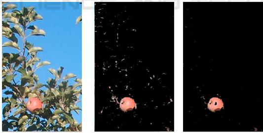
(a) Input image (b) After Hue segmentation (c) After Hue and Saturation segmentation
