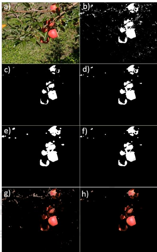
Figure 5: Stages of morphological operations (a) Original Image (b)Mask of pixel classification (c)Erosion (d) Dilatation (e) Dilatation (f) Erosion (g) RGB Mask of pixel classification (h) RGB Mask after applying morphological operations.
