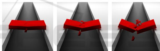
Figure 7: A brittle block collapses under its own weight.
