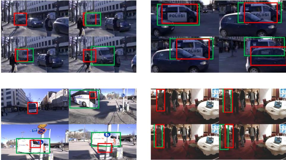
Figure 3: C-COT failures: (top left) the tracker bounding box was initialised to a region where the vehicle is occluded by trees/posts resulting to a wrong model learned (*noisy initialization*); (top right) the police car is occluded by another vehicle (*occlusion*); (bottom left) the bus is seen from the front, side and back view points with severe scale changes (*appearance change*); (bottom right) *other* reason for a tracking failure.
