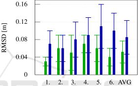
Figure 6: We compute the Root-Mean-Square Deviation in the x-y-plane between external tracking and onboard sensors. In "AVG" all six trajectories are averaged. Full results are shown in Table 2. For each scenario 10 trials were performed and values averaged.
