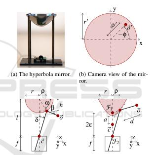
(c) Side view of spherical mir- (d) Side view of hyperbola ror.
