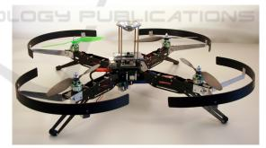
Figure 1: The quadrocopter utilized in this work. In the center, a camera captures omnidirectional images via the mounted mirror (Compare Fig. 3a).
