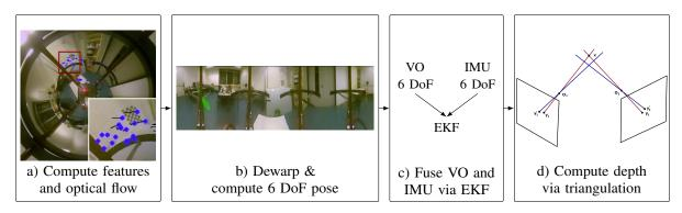
Figure 2: Pipeline of our proposed algorithm. a) Based on features we compute the optical flow. b) After dewarping the image, we estimate the pose change. c) An Extended Kalman Filter (EKF) combines the Visual Odometry (VO) results with values from the Inertial Measurement Unit (IMU). d) After having tracked features for multiple frames, we can estimate the point's depth using triangulation and build a depth map.
