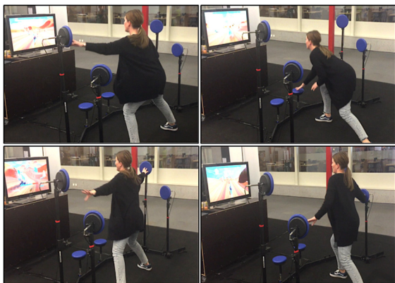
Figure 12: The new FBMC-setup allows for individual adjustments of height, distance and position of the but-tons.
