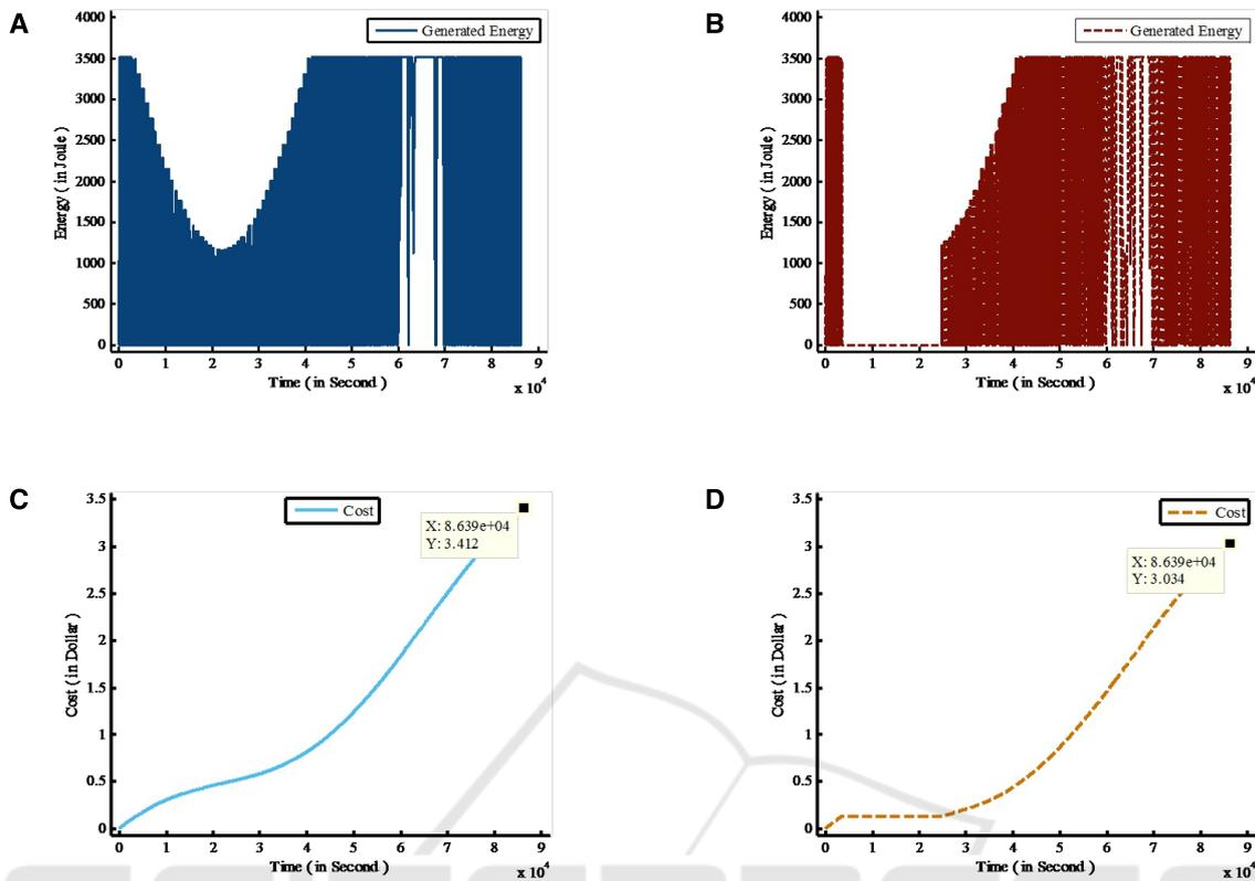
Figure 5: Simulation results. The first column corresponds to the presence of motion, whereas the second simulates the absence of motion. In each column, the rows from up to down show the amount of energy consumed by the controller and the corresponding total cost.
