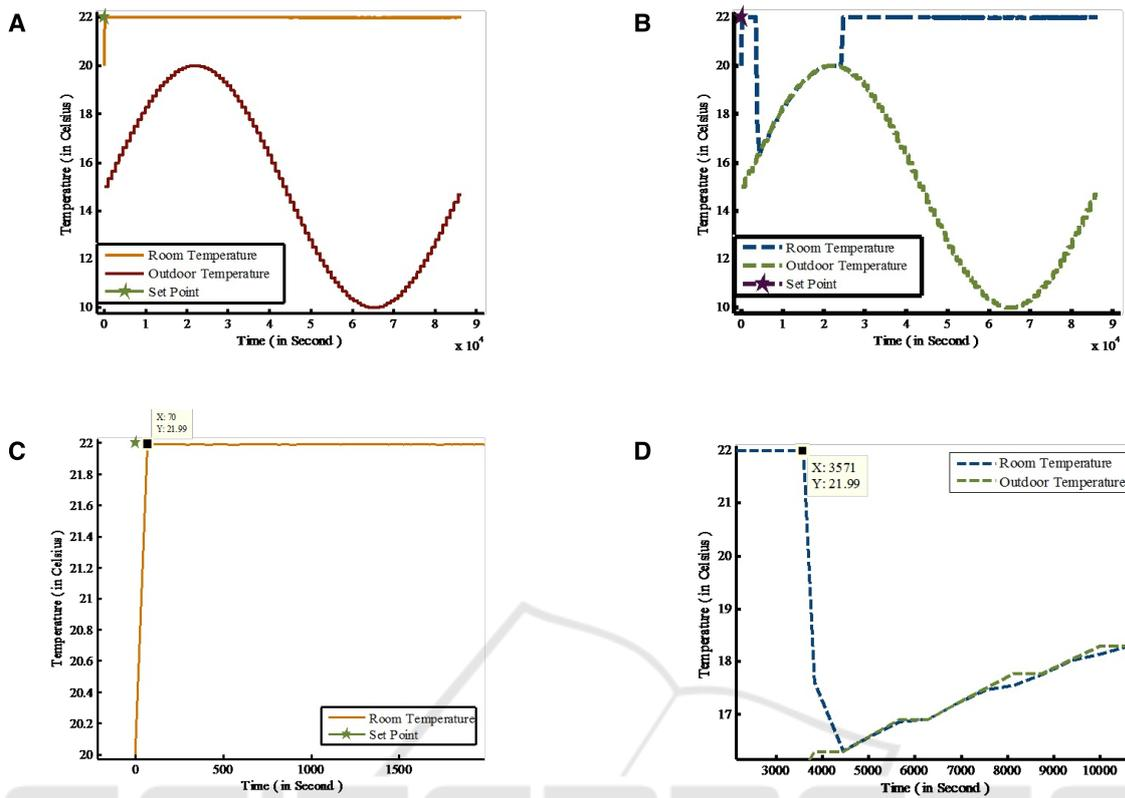
Figure 4: Simulation results. The first column corresponds to the presence of motion, whereas the second simulates the absence of motion. In each column, the rows from up to down show the neuro-fuzzy controller's output response and the controller's speed.
