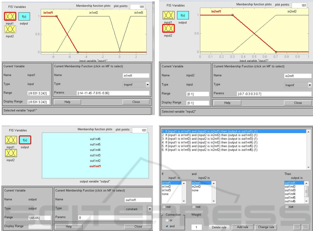
Figure 3: Modeling the Neuro-Fuzzy Controller with Matlab ANFIS toolbox.
