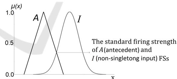
Figure 2: The *max* degree membership of the intersection between  $A$  (antecedent) and  $I$  (input) FSs is determined as firing strength which is an illustration of the standard approach in defining firing strength.
