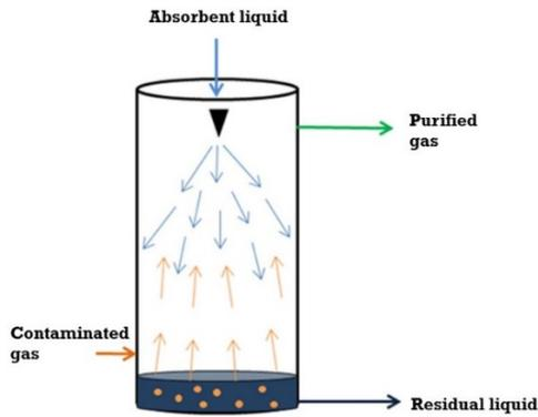
Figure 2: Spray column scheme.
