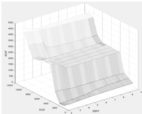
Figure 14: Simulation results of the SO<sub>2</sub>F for different values of SO<sub>2</sub>I (from 1000 to 11000 ppm<sub>v</sub>) and EBRT (from 2 to 10 seconds).
