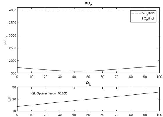
Figure 9:  $\text{SO}_2\text{F}$  prediction results obtained given an  $\text{SO}_2\text{I}$  value of 4000 ppm<sub>v</sub>, an EBRT of 0.8 seconds and different QL values.
