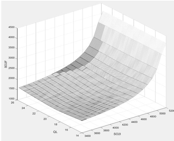
Figure 10: Simulation results of the SO<sub>2</sub>F for different values of SO<sub>2</sub>I (from 3400 to 5500ppm<sub>v</sub>) and QL (from 14 to 16 l/h).
