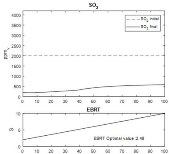
Figure 12: SO<sub>2</sub>F prediction results obtained given an SO<sub>2</sub>I value of 2000 ppm<sub>v</sub>, a QL of 18 l/h and different values of EBRT.
