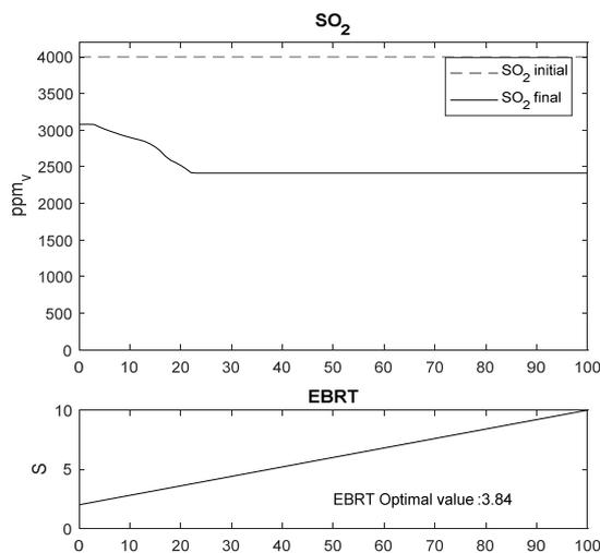
Figure 13: SO<sub>2</sub>F prediction results obtained given an SO<sub>2</sub>I value of 4000 ppm<sub>v</sub>, a QL of 18 l/h and different values of EBRT.
