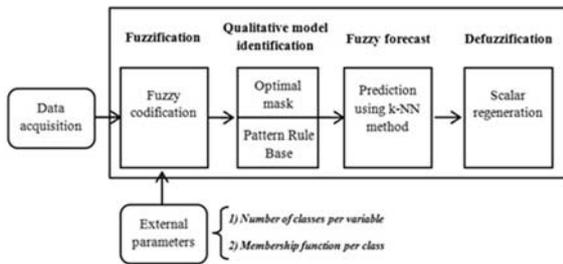
Figure 3: Schematic representation of the Fuzzy Inductive Reasoning (FIR) methodology.
