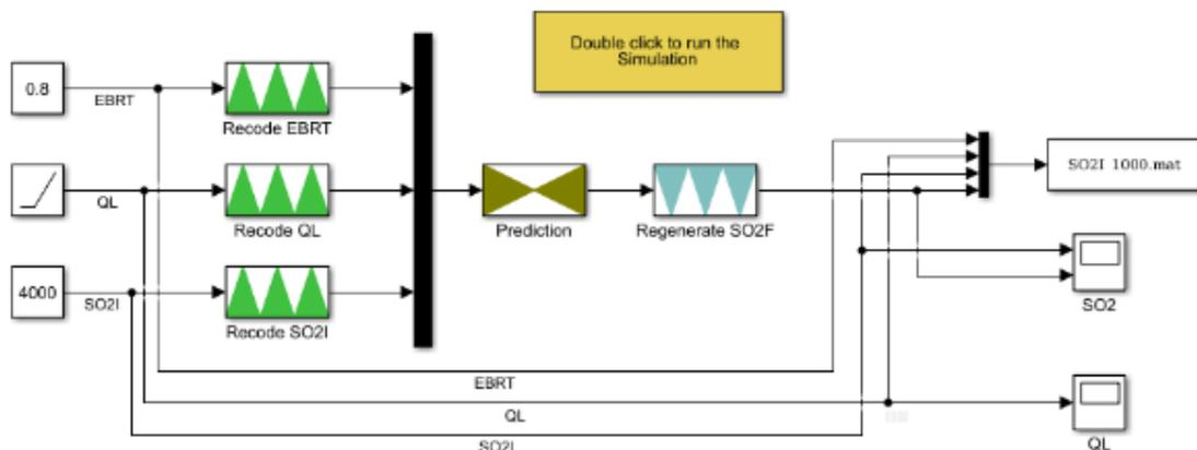
Figure 8: Simulation experiment of the amount of liquid injected into the plant using SIMULINK. EBRT, QL and  $\text{SO}_2\text{I}$  input variables are discretized by means of the recode function and the FIR prediction module is used to obtain the predicted values that are then regenerated by using the regeneration function of FIR.
