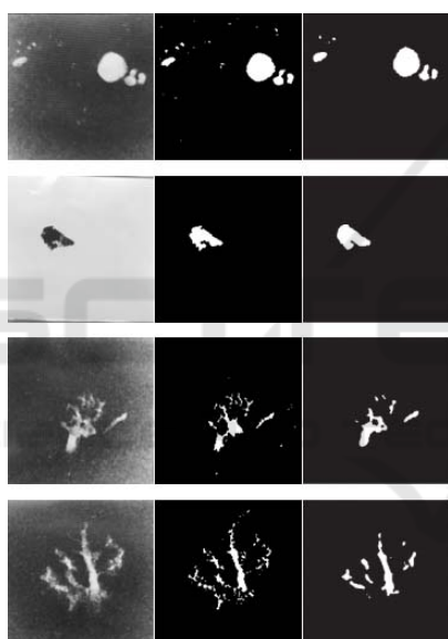
Figure 8: Illustration of comparative experiments between the proposed and Li's work: from the leftmost to the rightmost, the three columns are the original ASTM standard images, our results, Li's results.
