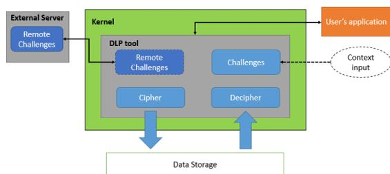
Figure 1: DLP tool architecture with server.
