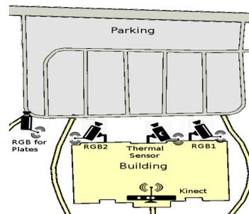
Figure 3: Outdoor Scenario and sensors positions.
