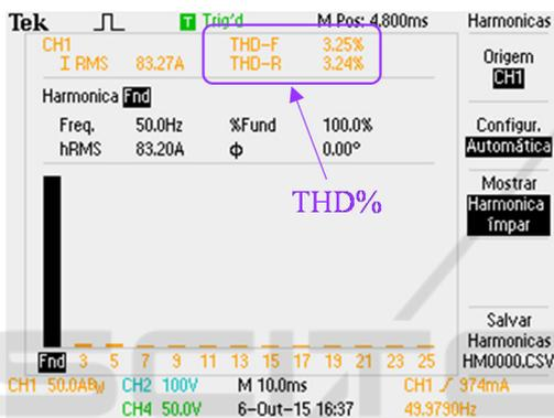
Figure 4: Experimental results of the traditional power factor correction topology: Harmonic spectrum of the grid current and measured THD%.
