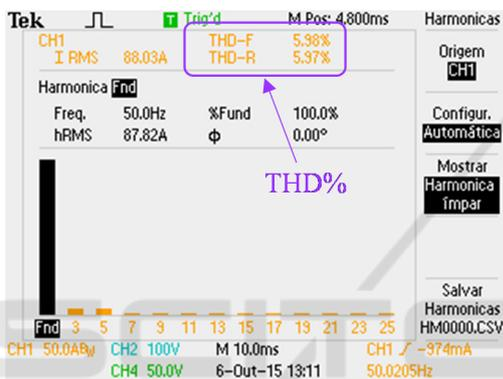
Figure 8: Experimental results of the asymmetrical bridgeless topology: Harmonic spectrum of the grid current and measured THD%.
