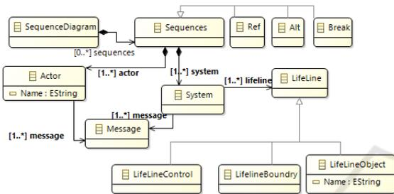
Figure 5: Main fragments of System Sequence Diagram Meta-model.
