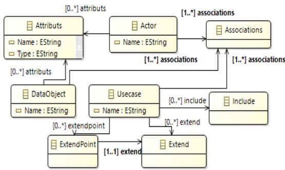
Figure 2: Main fragments of Use Case Diagram Meta-model.
