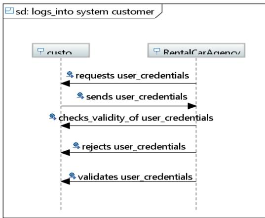
Figure 17: Generated "Authenticate" Sequence Diagram of RentalCarAgency.
