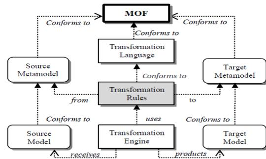
Figure 6: Relationship between the model transformation and meta-models.
