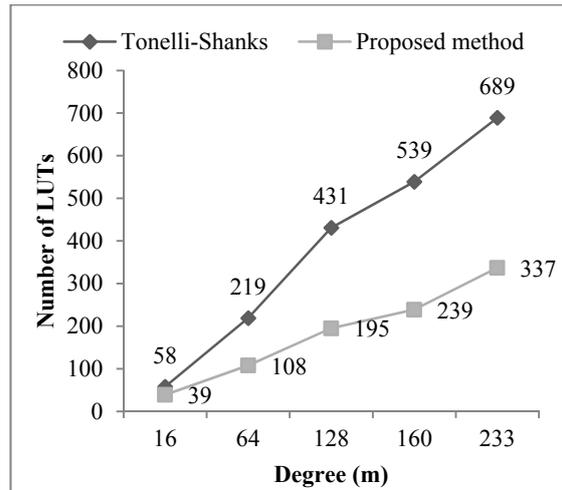
Figure 6: Number of LUTs needed in our method vs. Tonelli-Shanks algorithm.
