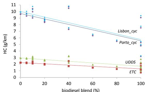
Figure 6: Engine HC emissions function of the biodiesel blend for the four simulated driving cycles.
