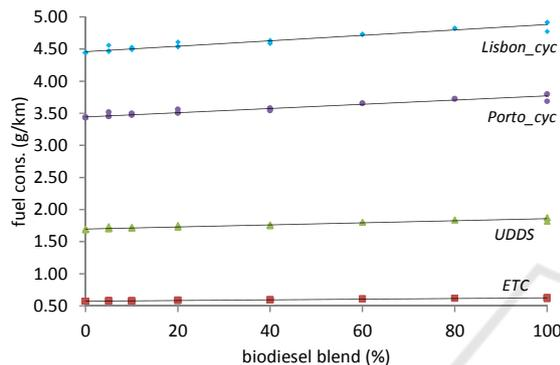
Figure 3: Engine fuel consumption function of the biodiesel blend for the four simulated driving cycles.
