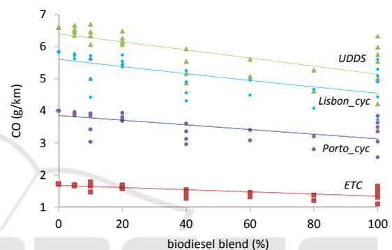
Figure 5: Engine CO emissions function of the biodiesel blend for the four simulated driving cycles.
