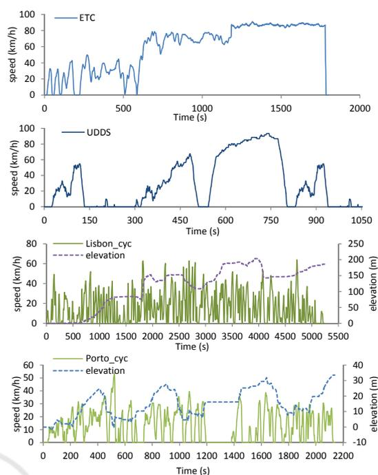
Figure 2: Driving cycles profile.
