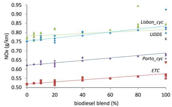
Figure 4: Engine NOx emissions function of the biodiesel blend for the four simulated driving cycles.
