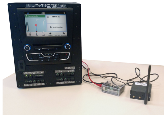
Figure 3: Implementation setup with the Ford TDK, a Raspberry Pi (a mini computer) and a cellular network router.
