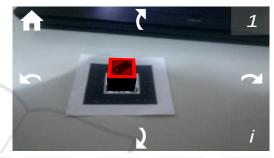
Figure 1: ARToolKit AR reader module, reading a paper marker.
