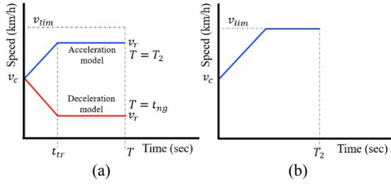
Figure 5: Acceleration/deceleration profile; (a): acceleration /deceleration to the recommended speed; (b): acceleration to the speed limit.
