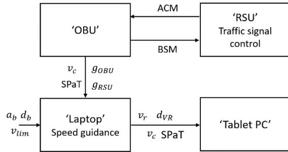
Figure 2: Flow chart of proposed eco-guidance system.
