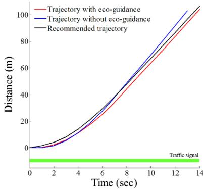
Figure 7: Time-moving distance graph in scenario 1.
