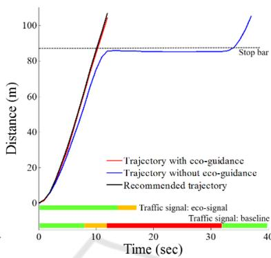
Figure 8: Time-moving distance graph in scenario 2.
