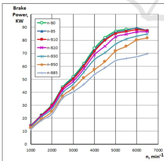
Figure 2: Influence of n-Butanol gasoline blended fuels on engine brake power.
