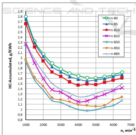
Figure 6: Influence of n-Butanol gasoline blended fuels on HC emissions.
