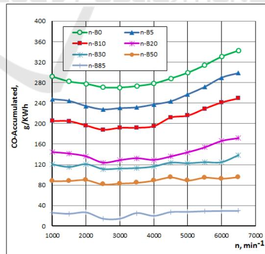
Figure 5: Influence of n-Butanol gasoline blended fuels on CO emissions.
