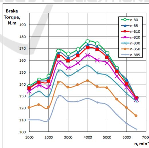
Figure 3: Influence of n-Butanol gasoline blended fuels on engine torque.
