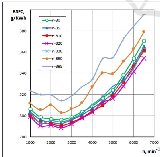
Figure 4: Influence of n-Butanol gasoline blended fuels on brake specific fuel consumption.
