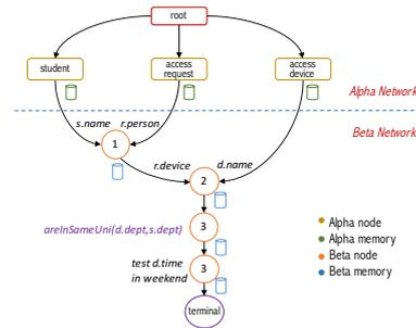
Figure 6: Rete graph for policy 1 with test expressions – A new node is added that checks compatibility of student and access device.
