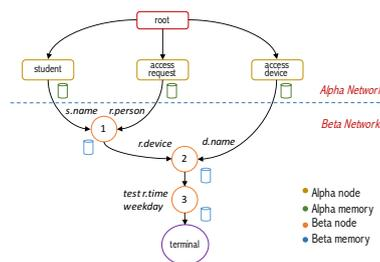
Figure 3: The Rete graph for classtime access rule – Once a token reaches the terminal node the rule is activated.
