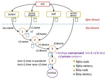
Figure 11: The scoped Rete graph for policy 3 – The expensive tests are replaced with scope tests performed by efficient encoding operations.
