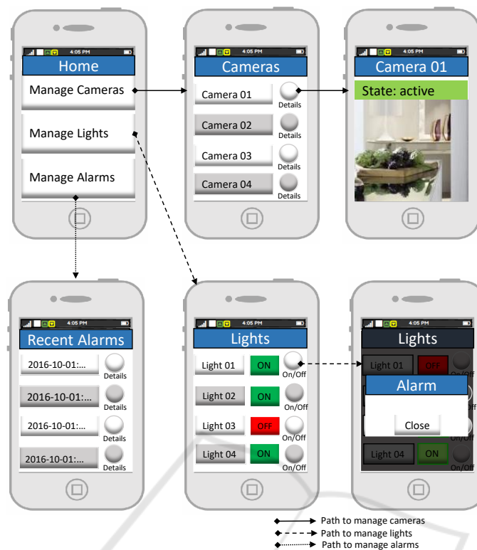
Figure 4: Case study: a piece of user interface of smart-house application.
