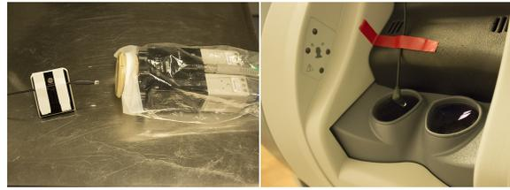
Figure 2: Test setup. Left: LED in front of endoscopic camera (without lens). Right: Light to voltage sensor in front of displays in the surgeon's console. Both were covered during measurements to block light from the environment.
