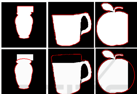
Figure 6: Segmentation results without shape prior (first row) and with shape prior (second row).
