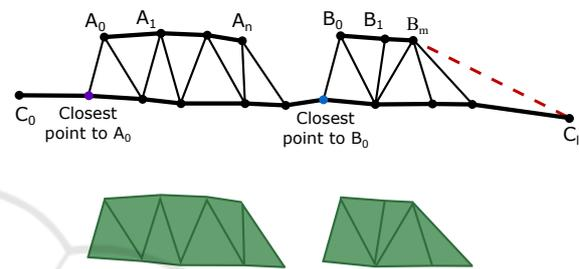
Figure 7: Top, example of a one-to-two triangulation of polylines using the proposed algorithm. Bottom, obtained triangles.
