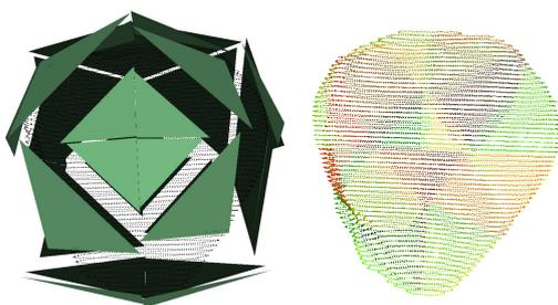
Figure 4: Left, a tetra-tree associated to the contour points. Right, points belonging to each tetra-cone are shown in a different colour.
