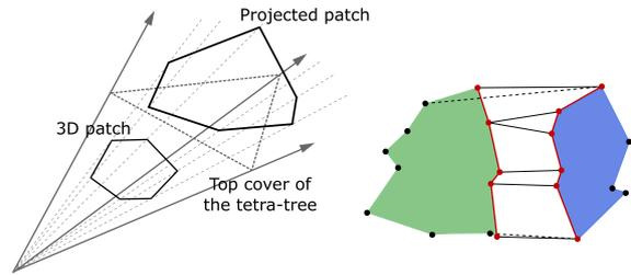
Figure 10: Left, schema that represents the linear projection of the external contours of a triangle patch onto the plane defined by the top cover of its associated tetra-cone. Right, schema representing the selection of the edges to be sewn between two patches. Solid lines connect points of edges that belong to the group of edges to be sewn group since they do not intersect with any patch. Dotted lines intersect with the patch, and therefore their associated edges are discarded.
