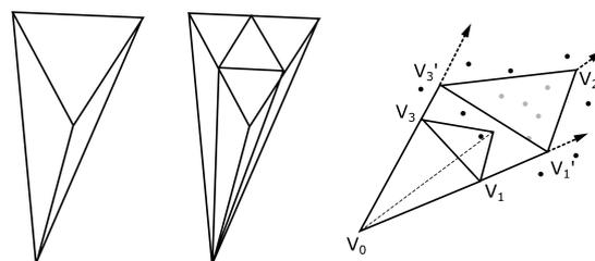
Figure 5: Left, a representation of the subdivision of a tetra-cone. Right, a schema that represents the bounding tetrahedra associated with a tetra-cone (Jiménez and Segura, 2008).
