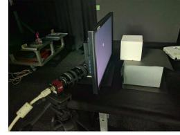
Figure 4: Display characteristics measurement: light source on the display moved, and changes of intensities on the cube were measured.
