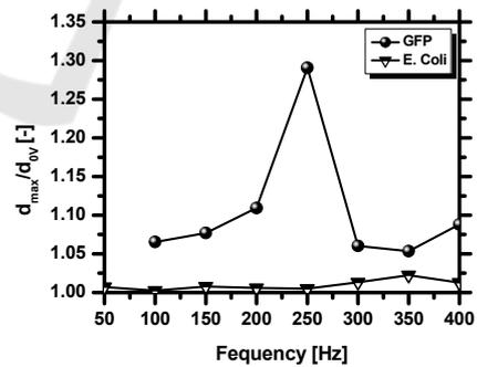
Figure 4: Maximum spreading dimensionless diameter of GFP ( $1.71 \times 10^{-3}$  mM) and GFP-expressing *E-coli* suspension ( $1 \times 10^9$  cells/mL), for droplets moving between coplanar electrodes (transport section of the device).
