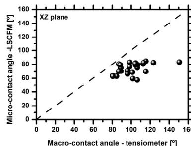
Figure 2: Comparison between the equilibrium angles measured with the optical tensiometer and with the LSCFM technique measured on micro-textured silicon wafer surfaces.
