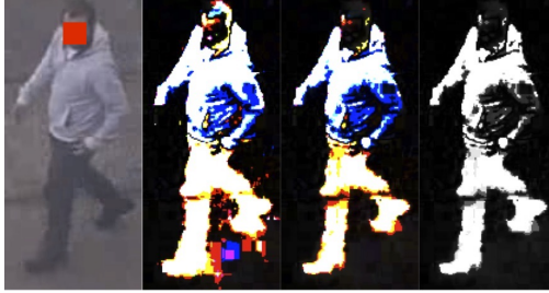
Figure 6: a) Original image, b) mask for \tau=20 , c) mask for \tau=30 and d) grayscale mask for \tau=30 .
