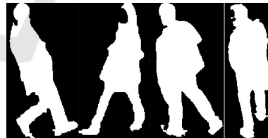
Figure 8: Example of human silhouettes using background subtraction combined with shadow and highlight removal.
