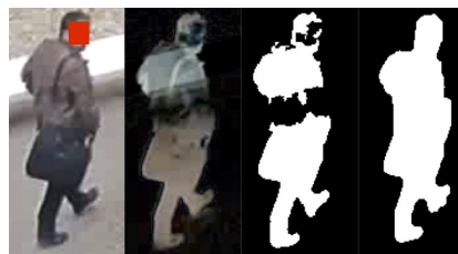
Figure 5: a) Original input image, b) result of absolute subtraction, c) binary image and d) result with shadow removal and highlight detection.
