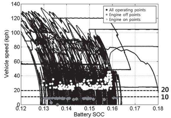
Figure 3: Points of engine turned on/off.
