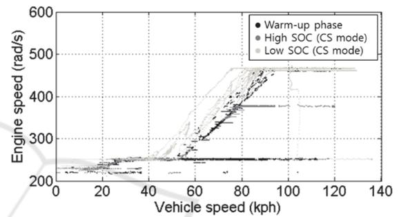
Figure 4: Engine speed vs. vehicle speed.
