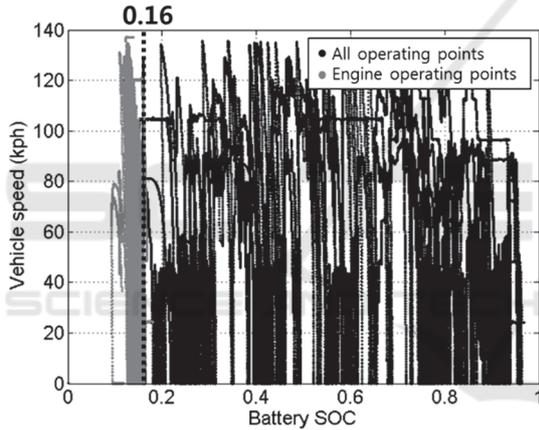
Figure 2: Vehicle and engine operating points.
