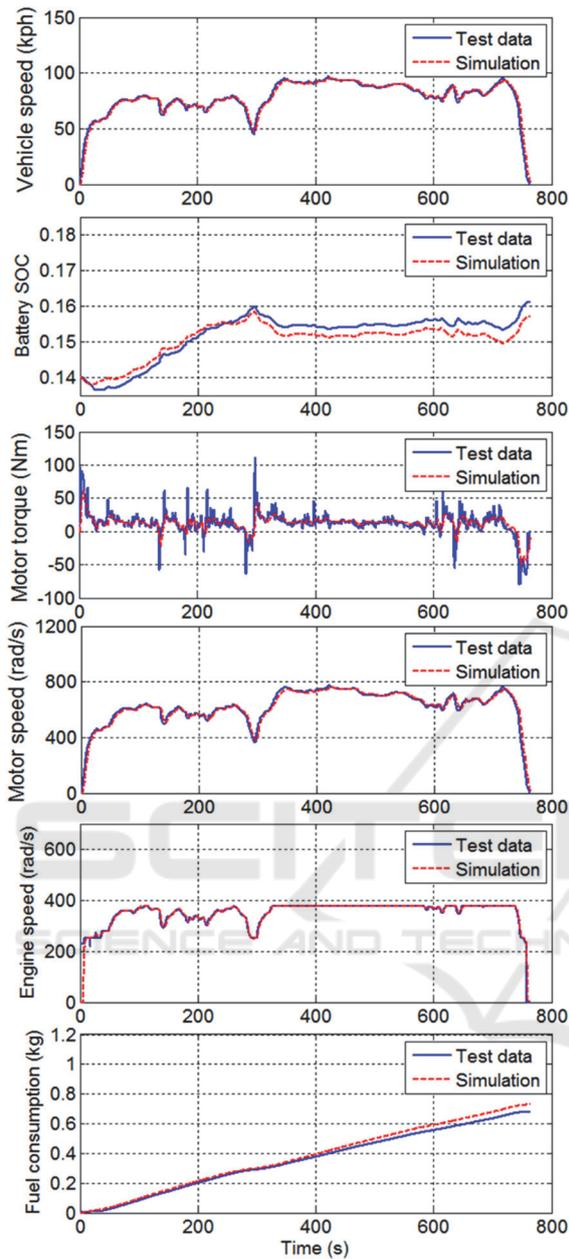
Figure 7: CS mode validation results for HWFET cycle.
