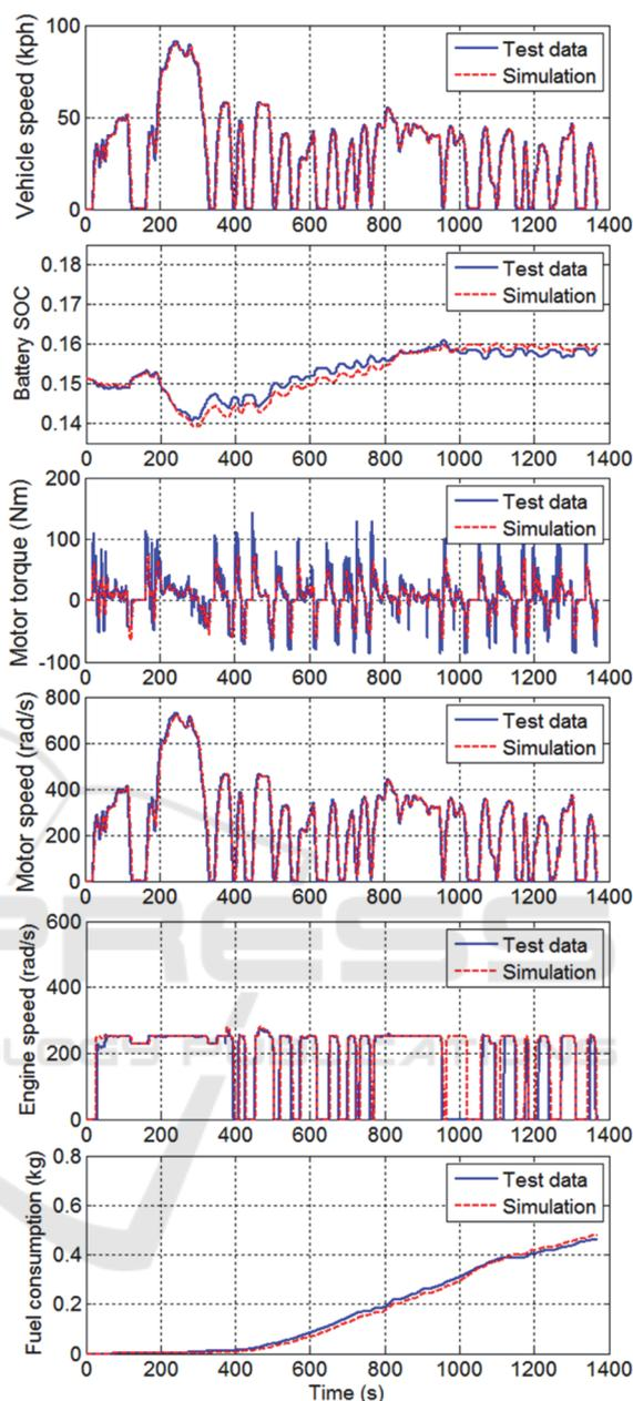
Figure 6: CS mode validation results for UDDS cycle.
