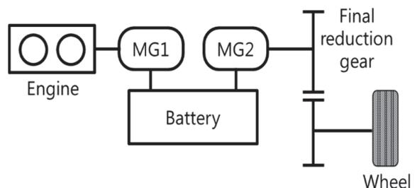
Figure 1: Vehicle configuration for RE-EV.
