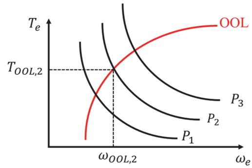
Figure 8: Determination of engine operating point in OOL control.
