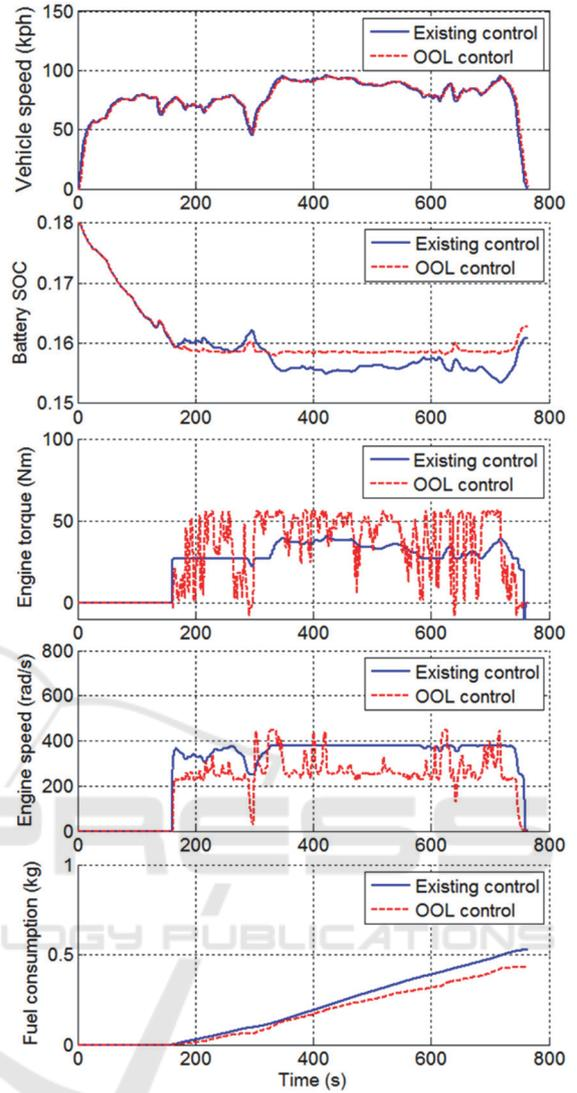
Figure 10: Simulation results for HWFET cycle.
