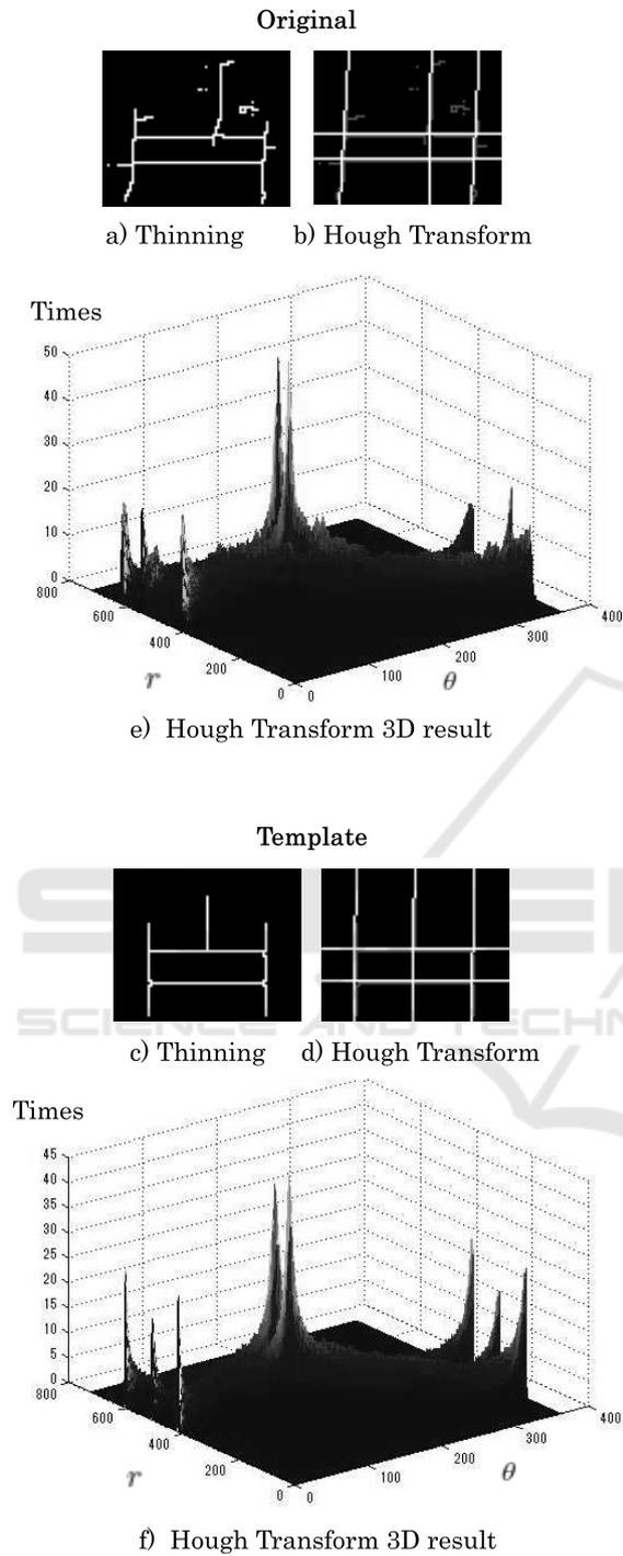
Figure 5: Hough transform.
