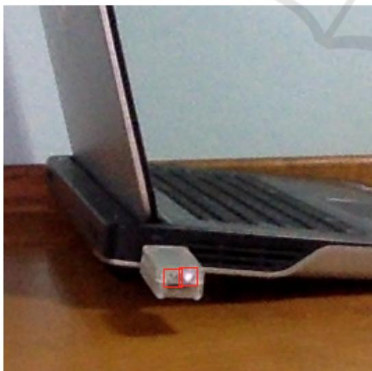
Figure 3: A screenshot of the exfiltration process after the handshake, as per the receiving view. The red rectangles show the location of each LED, only one is turned on in the picture, showcasing the distinctive color of infrared light.
