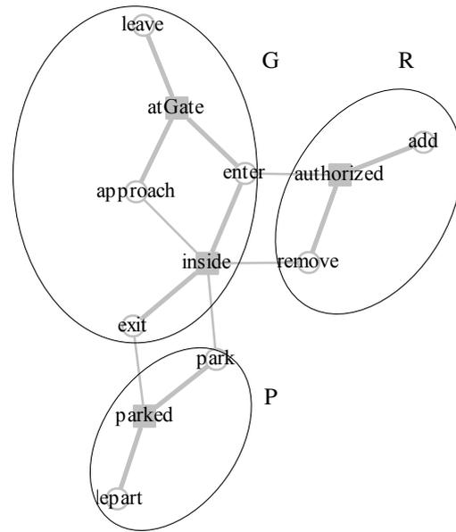
Figure 2: A dependency diagram of the parking lot with a suggested partition. Each subsystem candidate is enclosed in an ellipse. The edges that cross the partitions (when they exist) are few and weak. This partition corresponds to the decomposition in Section 3: (P) manages which car parks in which space, (R) manages the authorized list, and (G) manages the entry and exit to and from the parking lot.
