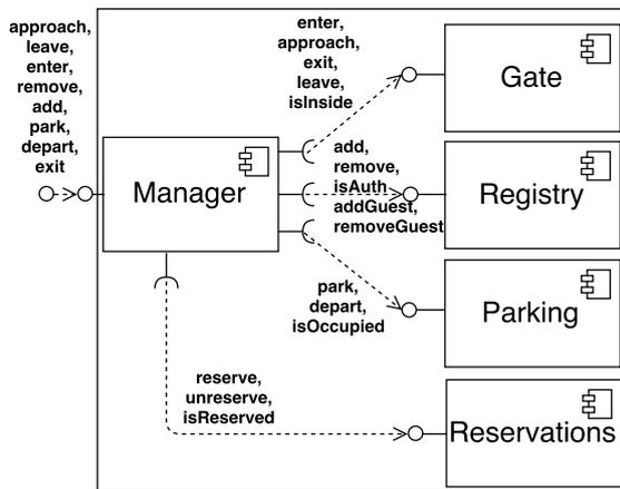
Figure 8: Component model of the evolved parking lot management system.
