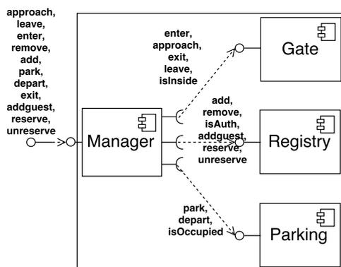
Figure 10: A revised component model of the evolved parking lot management system.
