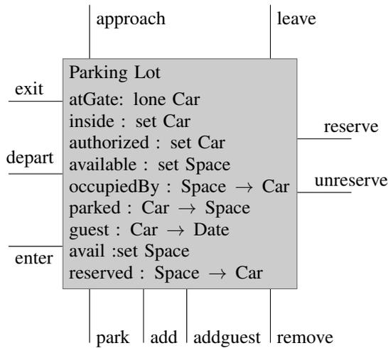
Figure 5: A subsystem diagram that summarizes the entire updated parking lot system. We have added operations for reserving parking spaces, and state variables that record guests and reserved parking spaces.
