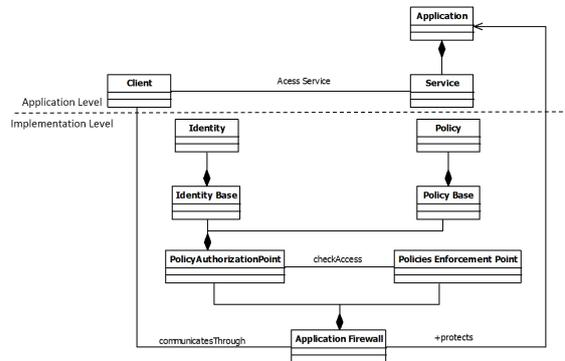
Figure 1: Application Firewall pattern.
