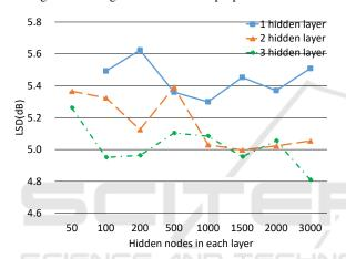
Figure 5: Change of LSD with a method to convert spectral envelope by DNN.
