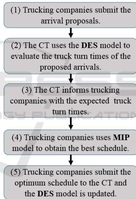
Figure 3: The operational steps of the proposed DCTAS.
