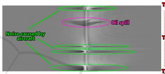
Figure 2: SLAR record representing a video sequence from time  $t_0$  to time  $t_n$  where  $t_i$  is considered an individual row of data. Oil slick is surrounded by purple and different noise patterns, because of the AV twists, by green.
