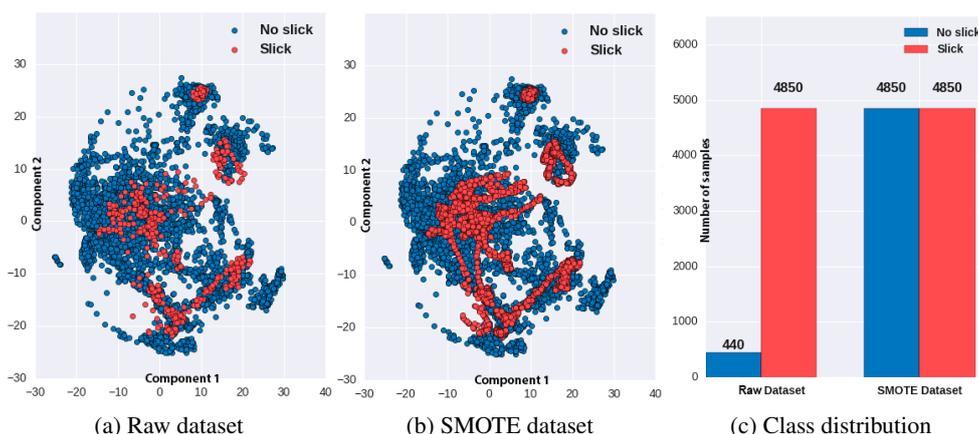
Figure 1: Sample distribution representation using Principal Component Analysis (PCA) (Jolliffe, 2002) over 1158 sized vectors of the original dataset and dataset with SMOTE.
