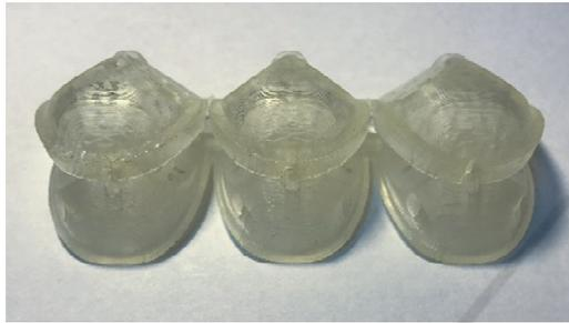
Figure 1: 3D Printed Resin Mold.
