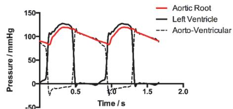
Figure 5: Time-varying pressure loadings measured in *in-vitro* experiment.
