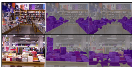
Figure 4: Qualitative Results: Our method is able to detect clutter in case of cluttered indoor scenes where support structures are not visible. The 2nd and 3rd columns shows the ground-truth labelling and our method labelling respectively(Figure best viewed in color and enlarged).
