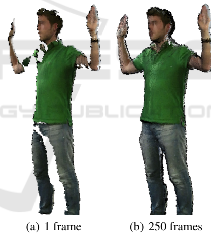
Figure 1: In this paper, we propose a non-rigid reconstruction pipeline for human body reconstruction. While parts of the body can move up to 5cm during capturing, the reconstruction stays rigid.
