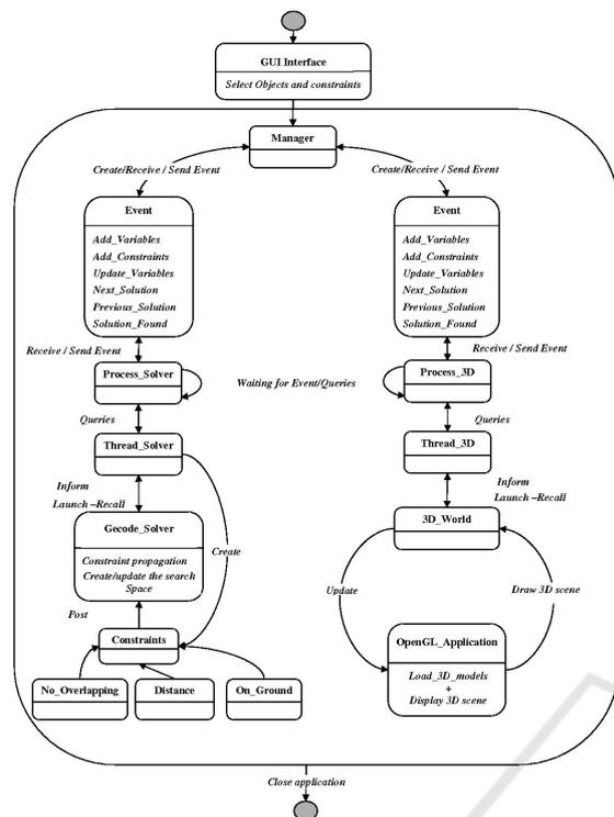
Figure 1: System architecture (event exchange between VE and Solver).
