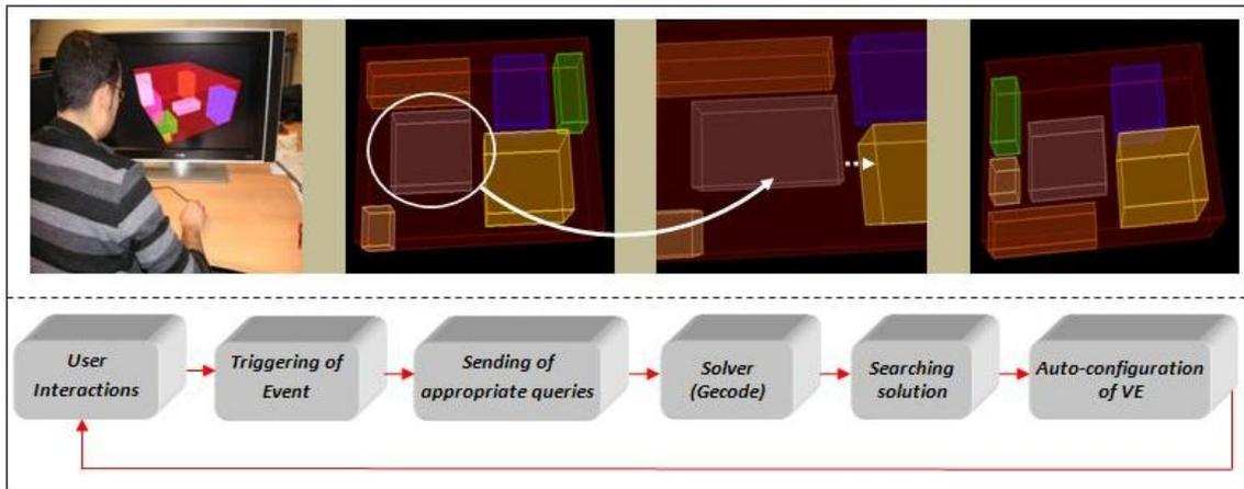
Figure 3: Illustration of the rearrangement of the 3D scene according to an object displacing.
