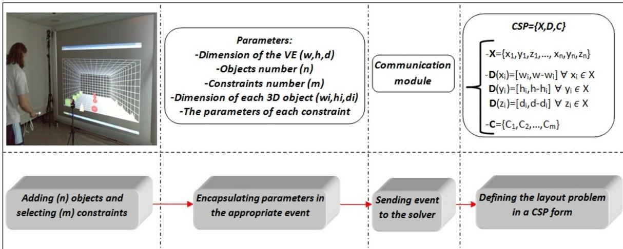
Figure 2: Architecture of the system.
