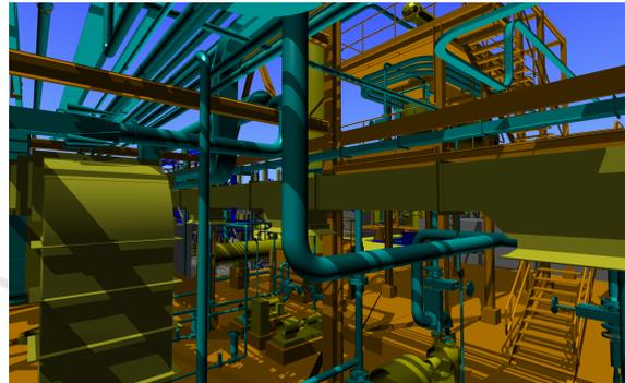
Figure 6: Close up view of the plant model. The intricate structure is modeled with the primitives described in the AVEVA RVM CAD format.
