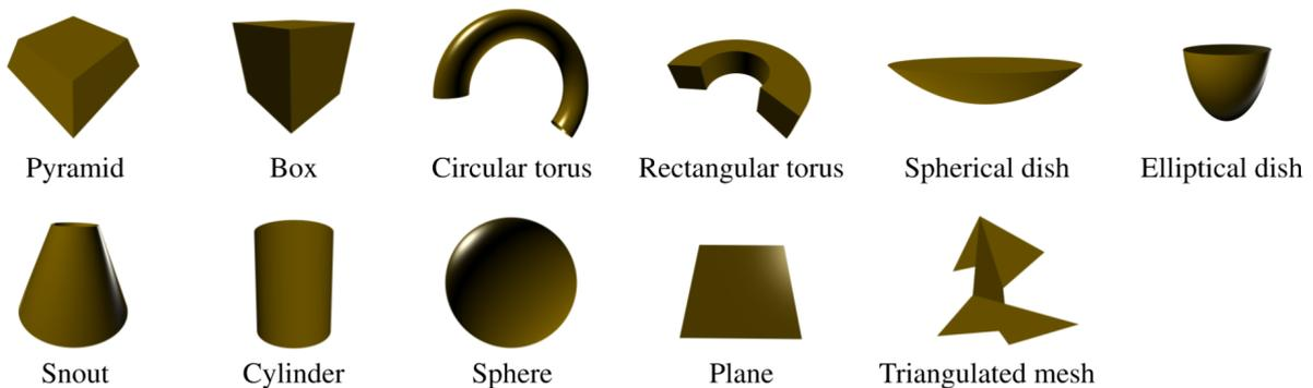
Figure 4: RVM primitives used in the plant model.
