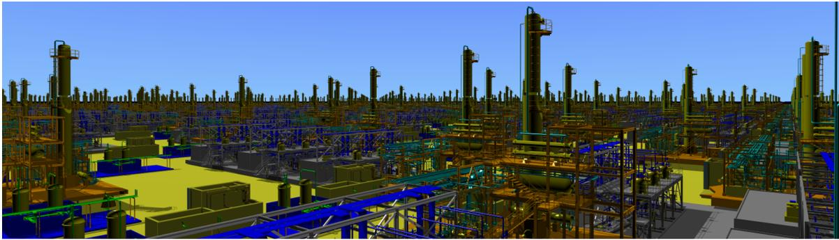
Figure 1: A complex CAD scene built out of 8,000 individual plant models. In total, the scene consists of more than 100,000,000 non-planar second-order (cylinders, cones, etc.) and fourth-order (tori) primitives, ray traced at more than 10 frames per second on 16 CPU cores, including pixel-accurate shadows.
