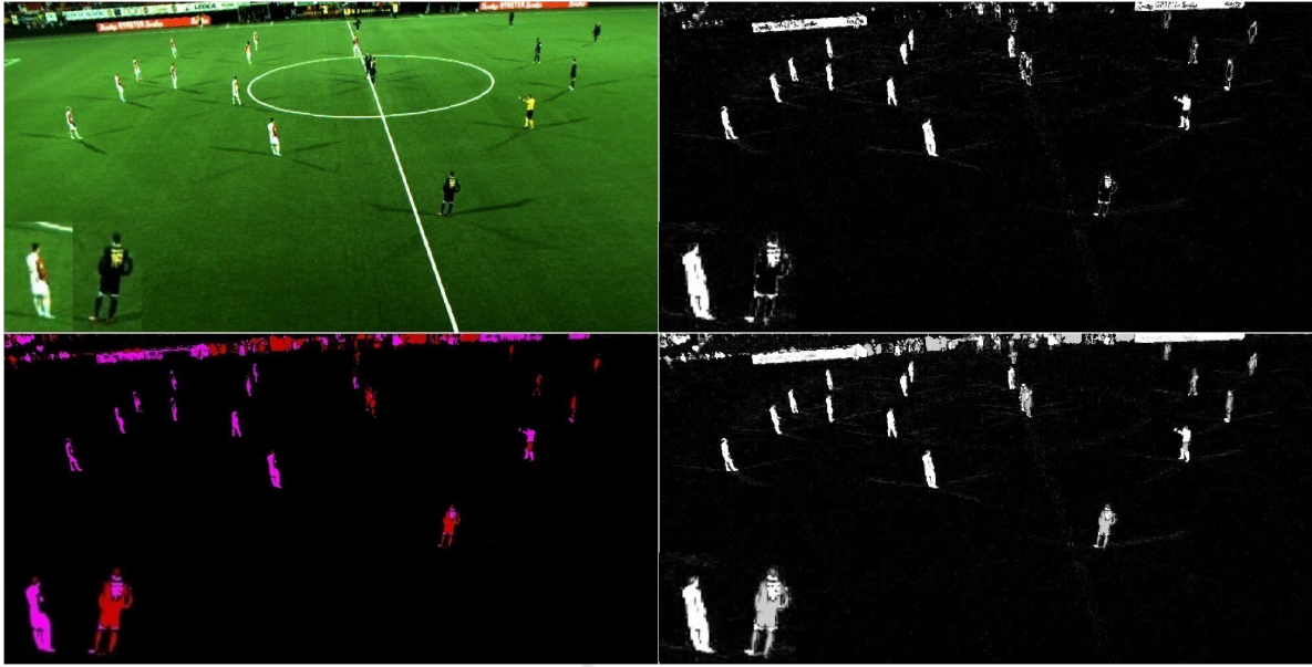
Figure 5: Top-left: Input frame, top-right: foreground objects identified due to high system error, bottom-left: foreground objects identified due to abnormally low (red) or high(magenta) visibility values, bottom-right: final result. A player from each team is shown magnified in the bottom-left of each sub-image.
