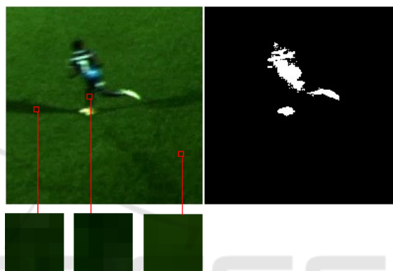
Figure 10: A failure case. Motion blur causes parts of the player to match regions in shadow which causes misidentification.
