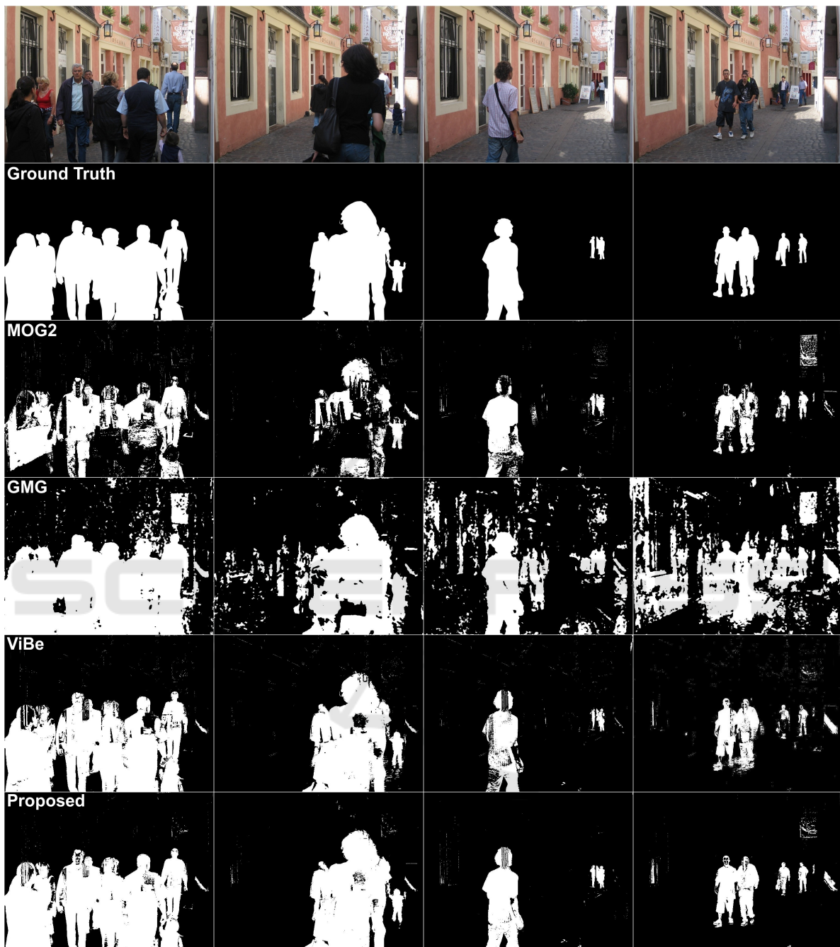
Figure 8: Comparison of MOG2, GMG, ViBe and our method for a scene with pedestrians.
