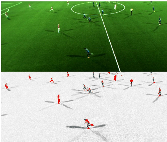
Figure 2: Video frame (above) and computed visibility (below) according to Equation (6). Red indicates visibility values greater than one.
