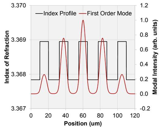
Figure 2: A structure useful for demonstrating the effects of changes to the index profile.
