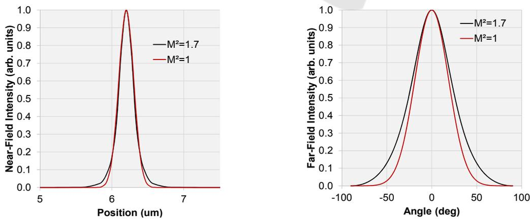
Figure 6: Near-field (left) and far-field (right) intensity distributions for an engineered structure with  $M^2$  of 1.7 and 86 percent of its power in the far-field within the diffraction limit.
